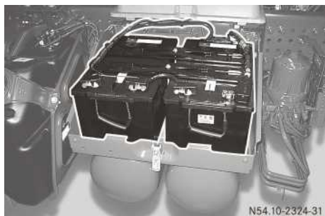
Example: batteries on the side on the chassis, one beside the other
