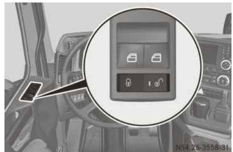
Door control panel (example: left-hand door)
