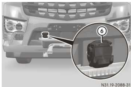
Example: duomatic coupling, front
