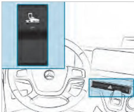
In road paver mode, the level control system permanently regulates the driving level, regardless of operating conditions. This enables the level relative to the road paver mode to be maintained and forced lowering is deactivated.
