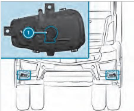
Front fog lamp (example: front fog lamp with LED daytime running lamp in the Arocs)
