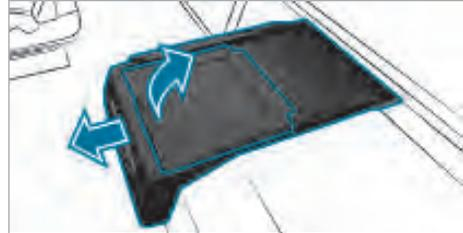
The drawer under the berth can also be equipped with a refrigerator box. You can find notes on using and adjusting the refrigerator box in the separate Owner's Manual.
