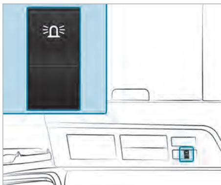
Rotating beacon button in the overhead control panel (example)
