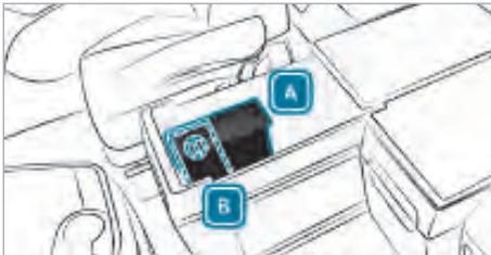
▶ Use the waste receptacle only in position **A** or **B**. Otherwise, the waste receptacle will not be secured and may tip over during a journey.
