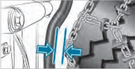
**!** **NOTE** Damage to the steering linkage due to snow chains
