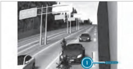
After switching on the ignition or after changing the semitrailer/trailer, adjustable distance line **1** shown in the display can be moved to the back edge of the trailer/semitrailer.
