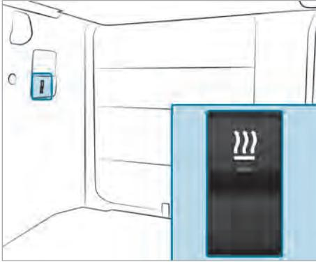
Additional button on the bed/berth switch panel (example: vehicle without stationary air conditioning system)
