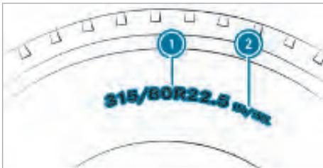
Example: tyre size and load-bearing index
